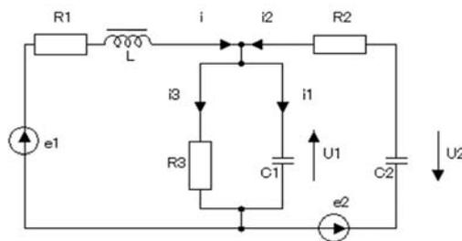
Fig. 7. The electrical circuit with a nonlinear coil [15]
