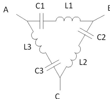
Fig. 8. Connection diagram of the tested capacitor bank and the choke
