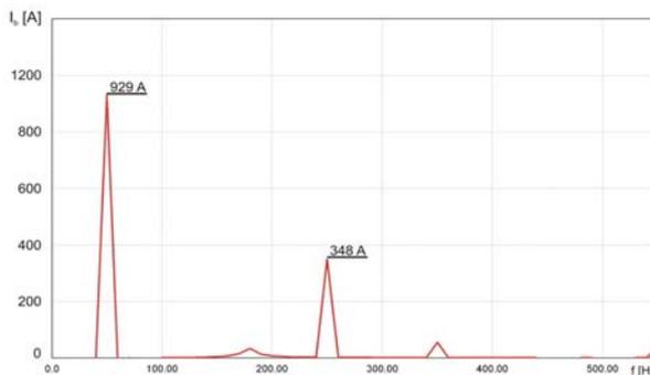
Fig. 13. Simulation of the 1<sup>st</sup> and 5<sup>th</sup> harmonic currents in a new capacitor bank
