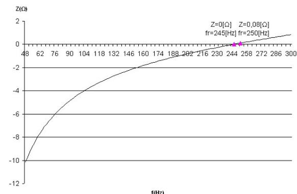
Fig. 11. Z(f) parameter for a 80kvar (400V) step of an old capacitor bank
