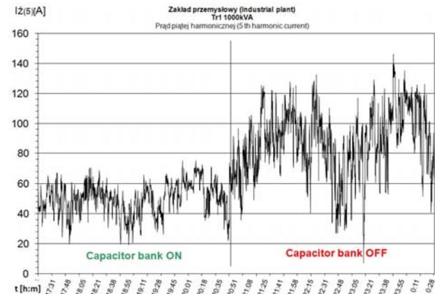
Fig. 4. Graph of a selected voltage harmonic measured at point A with a capacitor bank on and off
