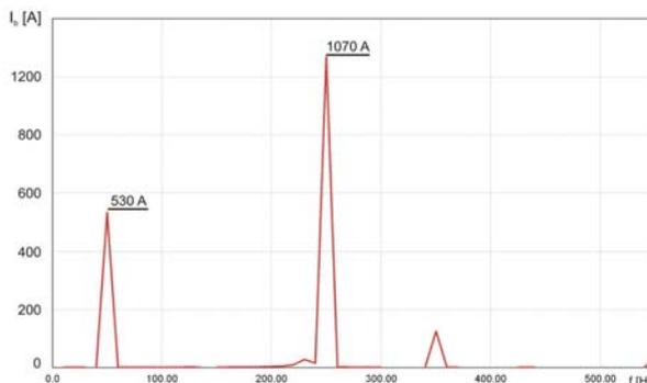
Fig. 14. Simulation of the 1st and 5th harmonic currents in a worn-out capacitor bank
