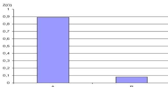
Fig. 12. Comparison graph of 5<sup>th</sup> harmonic impedance of a new (A) and worn-out (B) step of a capacitor bank
