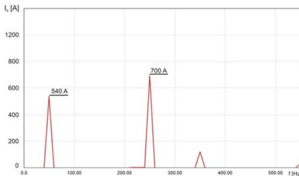
Fig.15. Current  $I_F$  in a passive 5<sup>th</sup> harmonic filter for the 1<sup>st</sup> and 5<sup>th</sup> harmonics (simulation) with a worn-out capacitor bank connected to the network
