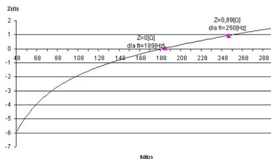
Fig. 9. Z (f) parameter for a 80kvar (400V) step of a brand-new capacitor bank
