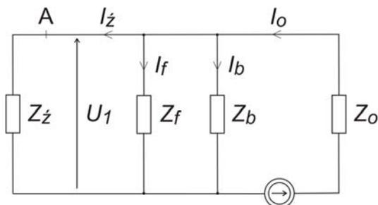
where:  $Z_z$  – power source impedance,  $Z_f$  – filter impedance,  $Z_b$  – capacitor bank impedance,  $Z_o$  – current source impedance.
