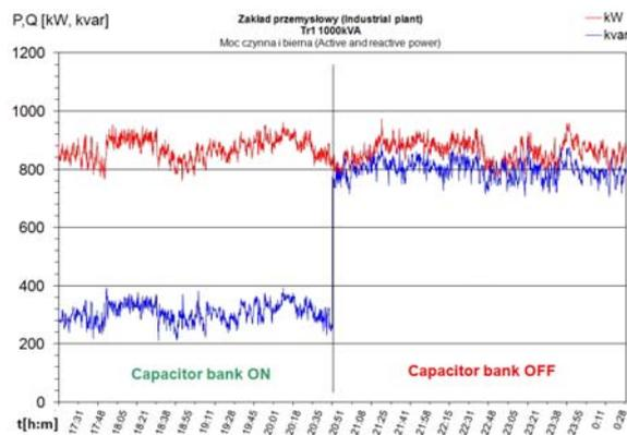
Fig. 2. Active and reactive power graphs with a reactive power compensation unit correspondingly off and on
