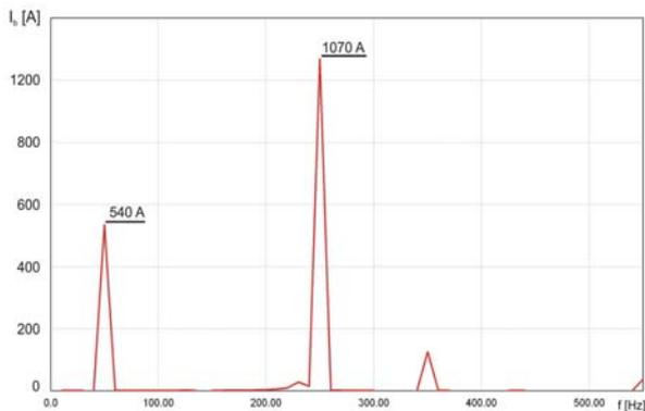
Fig.16. Current  $I_F$  in a passive 5<sup>th</sup> harmonic filter for the 1<sup>st</sup> and 5<sup>th</sup> harmonics (simulation) with a worn-out capacitor bank disconnected from the network
