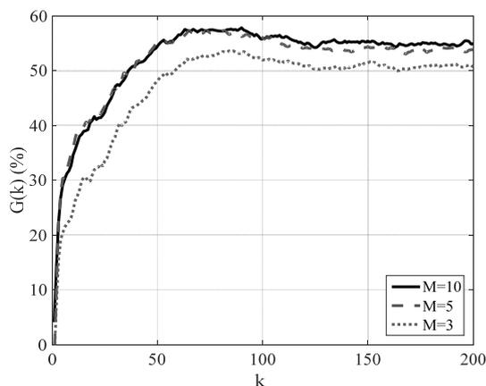
Fig.8.  $G(k)$  of estimation in a case of log-normal distribution of  $R(k)$  for various  $M$
