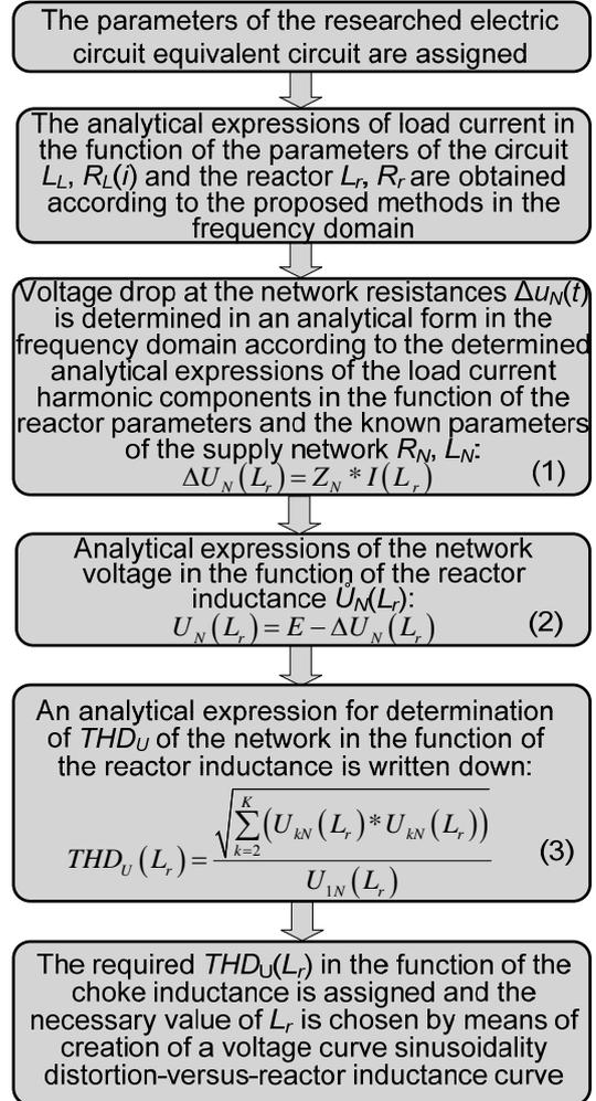
Fig. 3. Algorithm of the calculation and choice of the linear reactor
