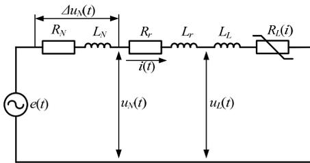
Fig. 2. Equivalent circuit of the electricity supply network section with a nonlinear load
