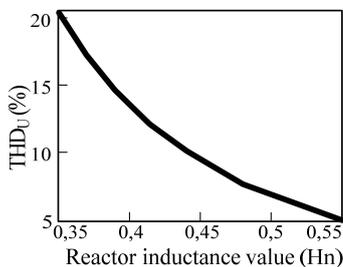
Fig. 4.  $THD_U$  versus reactor inductance  $L_r$  curve
