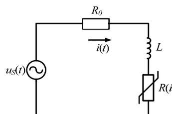
Fig. 1. Electric circuit with an active-inductive load
