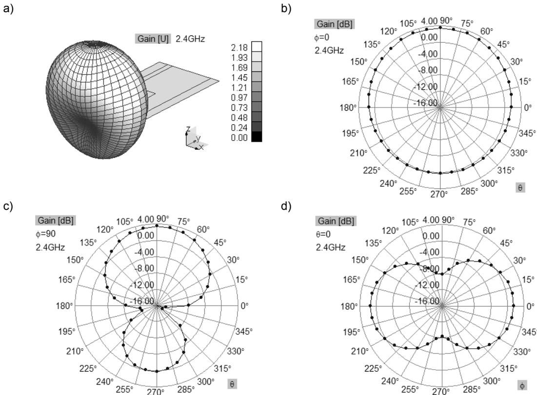
Fig.3. 3D radiation pattern of the antenna at 2,4 GHz operation band in a linear scale (a) and the main cross-sections of radiation patterns of the antenna: x-z plane (b), y-z plane (c) and x-y plane (d)
