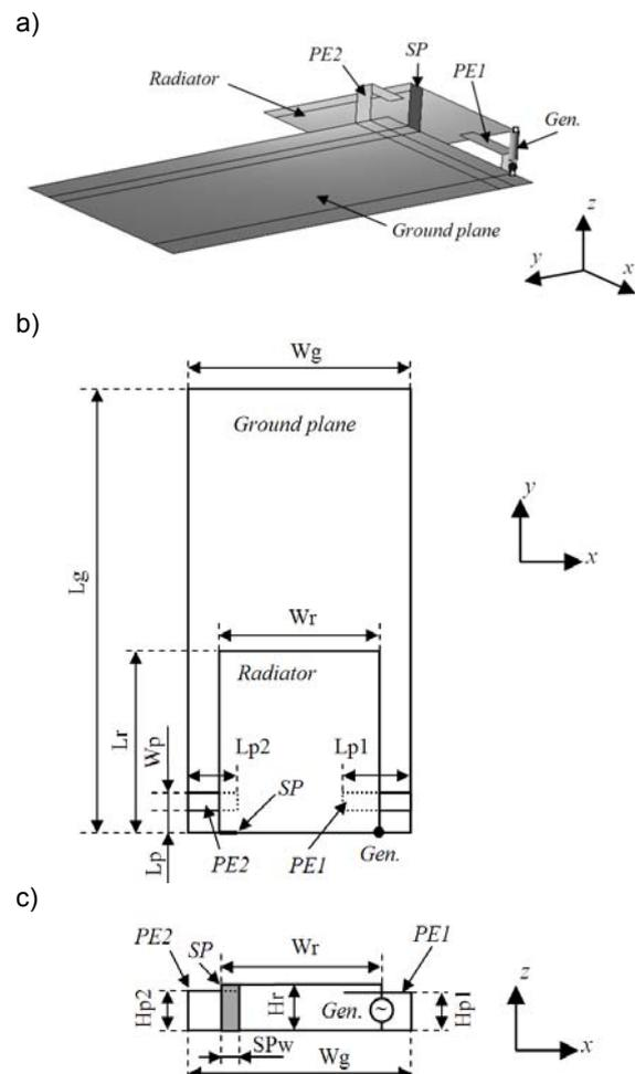
Fig.1. The structure of the analyzed antenna: an overall view from the bottom of the antenna (a) and the projection on x-y plane (b) and x-z plane (c)
