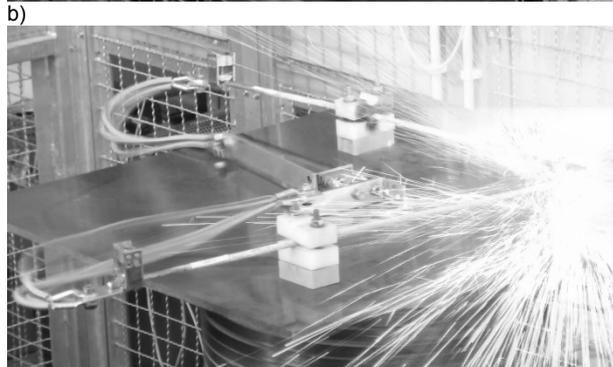
Fig. 4 Cross connector before the tests (a) and during the test (b) with 100 kA current and shape 10/350  $\mu$ s
