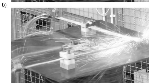
Fig. 6 Cross flat connector before the test (a) and during the test (b) with 100 kA current and shape 10/350  $\mu$ s
