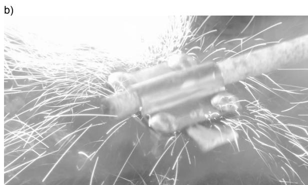
Fig.9 Cross connector assembled before the test (a), during the test (b) with 100 kA current and shape 10/350  $\mu$ s
