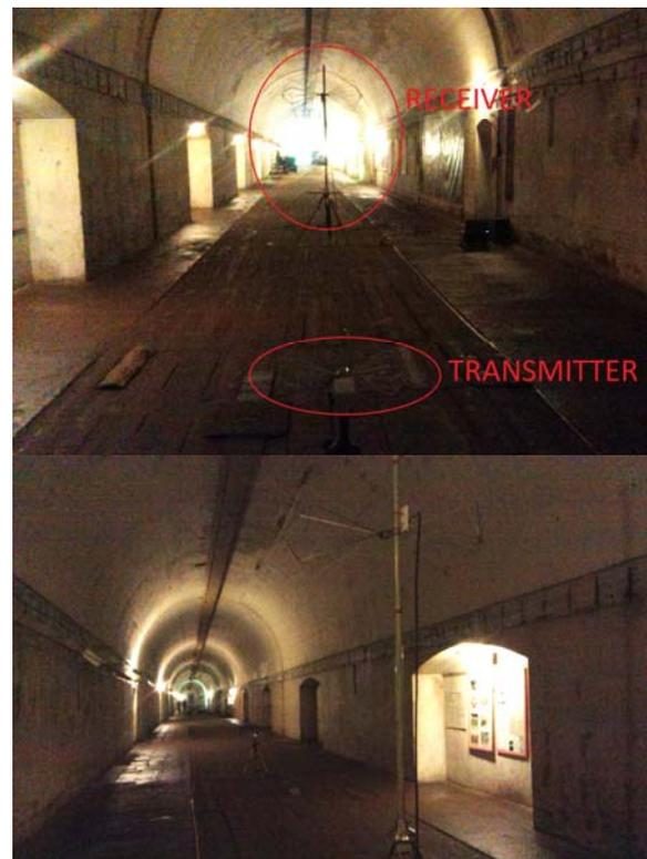
Fig 5. Test set-up inside the tunnel
