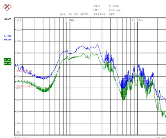
Fig. 3. Example of conducted disturbances from the locomotive, measured in catenary.
