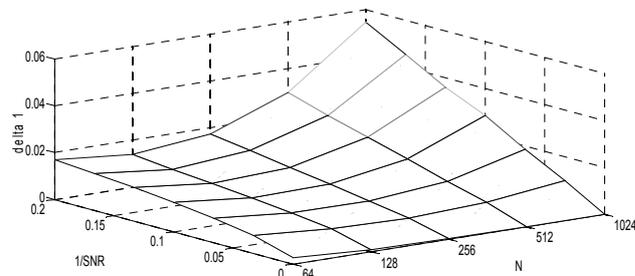
Fig. 15. Dependence of error  $\delta_1$  on  $N$  and  $1/SNR$ , for triangular signal,  $M=100$ ,  $\delta f = \delta T_d = 10^{-6}$
