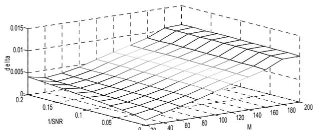
Fig.5. Dependence of error  $\delta$  for 1<sup>st</sup> harmonic on  $M$  and  $1/SNR$ ,  $N=256$ ,  $\delta f = \delta T_d = 10^{-6}$
