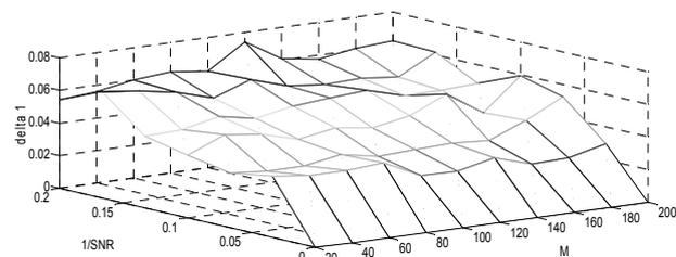
Fig. 16. Dependence of error  $\delta_1$  on  $M$  and  $1/SNR$ , for triangular signal,  $N=256$ ,  $\delta f = \delta T_d = 10^{-6}$
