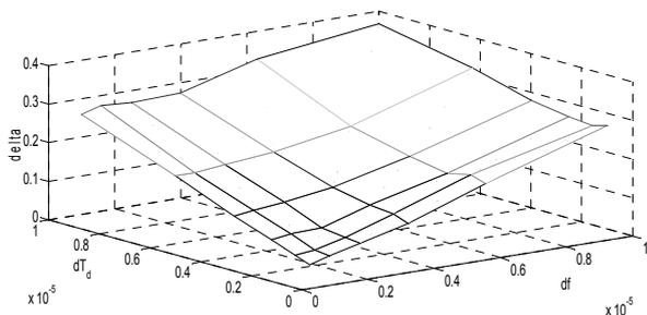
Fig. 10. Dependence of error  $\delta$  for 5<sup>th</sup> harmonic on  $\delta f$  and  $\delta T_d$ ,  $N=256$ ,  $M=100$ ,  $1/SNR=0,1$
