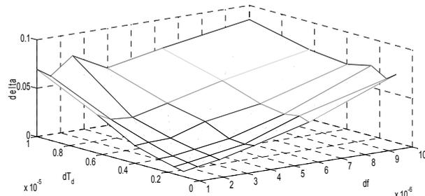
Fig. 9. Dependence of error  $\delta$  for 1<sup>st</sup> harmonic on  $\delta f$  and  $\delta T_d$ ,  $N = 256$ ,  $M=100$ ,  $1/SNR=0,1$
