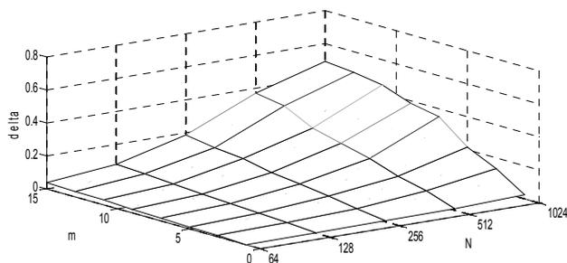
Fig. 2. Dependence of error  $\delta$  on  $m$  and  $N$ ,  $M = 100$ ,  $1/SNR = 0,1$ ,  $\delta f = \delta T_d = 10^{-6}$
