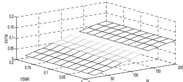
Fig.6. Dependence of error  $\delta$  for 5<sup>th</sup> harmonic on  $M$  and  $1/SNR$ ,  $N=256$ ,  $\delta f = \delta T_d = 10^{-6}$
