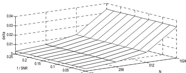
Fig.3. Dependence of error  $\delta$  for 1<sup>st</sup> harmonic on  $N$  and  $1/SNR$ ,  $M=100$ ,  $\delta f = \delta T_d = 10^{-6}$
