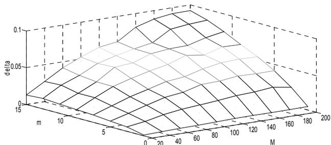
Fig. 1. Dependence of error  $\delta$  on  $m$  and  $M$ ,  $N = 256$ ,  $1/SNR = 0,1$ ,  $\delta f = \delta T_d = 10^{-6}$
