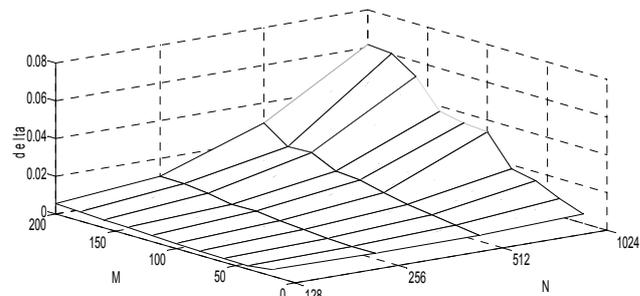
Fig. 7. Dependence of error  $\delta$  for 1<sup>st</sup> harmonic on  $N$  and  $M$ ,  $1/SNR=0,1$ ,  $\delta f = \delta T_d = 10^{-6}$
