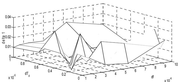
Fig. 11. Dependence of error  $\delta_1$  on  $\delta f$  and  $\delta T_d$  for triangular signal,  $N=256$ ,  $M=100$ ,  $1/SNR=0$
