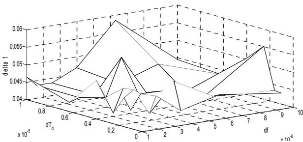
Fig. 12. Dependence of error  $\delta_1$  on  $\delta f$  and  $\delta T_d$  for triangular signal,  $N=256$ ,  $M=100$ ,  $1/SNR=0,1$
