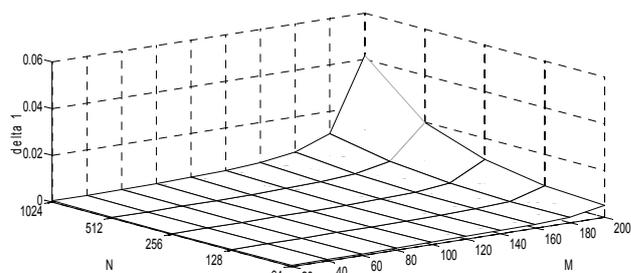
Fig. 14. Dependence of error  $\delta_1$  on  $N$  and  $M$  for triangular signal,  $\delta f = \delta T_d = 10^{-6}$ ,  $1/SNR=0,1$
