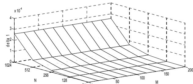
Fig. 13. Dependence of error  $\delta_1$  on  $N$  and  $M$  for triangular signal,  $\delta f = \delta T_d = 10^{-6}$ ,  $1/SNR=0$
