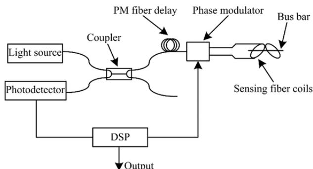
Fig. 7. Basic scheme of principle of S-FOCS.
