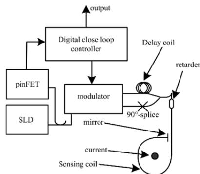
Fig. 4. Basic scheme of FOCS without FPR.
