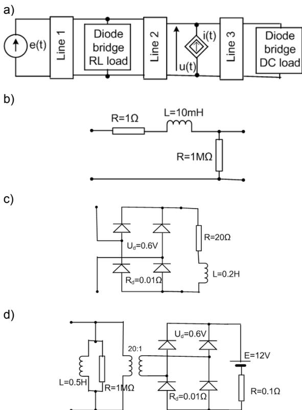
Fig. 5. Simulated circuit, a) structure, b) lines, c) load 1, d) load 2
