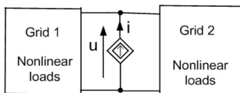
Fig. 1. General structure of voltage-controlled single-phase shunt active filter
