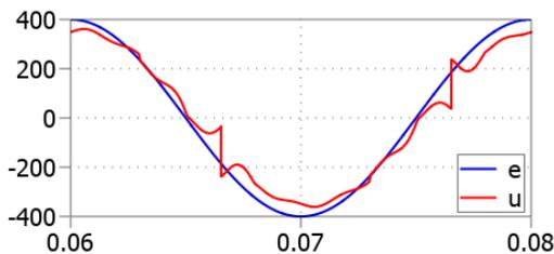
Fig. 8. Voltage waveform of the generator and voltage at the compensator location after compensation
