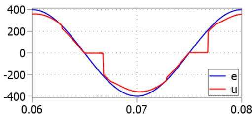
Fig. 7. Voltage waveform of the generator and voltage at the compensator location before compensation
