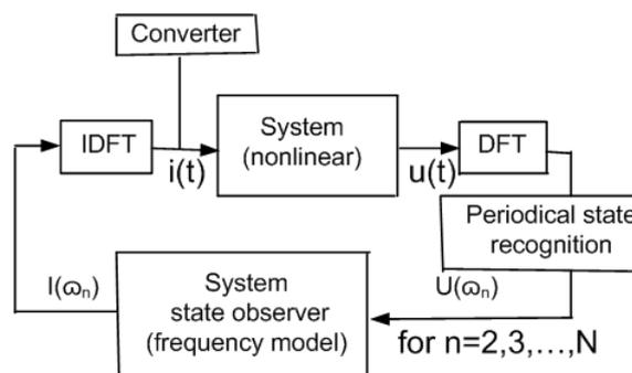
Fig. 2. Block diagram for searching of reference signal  $i(t)$
