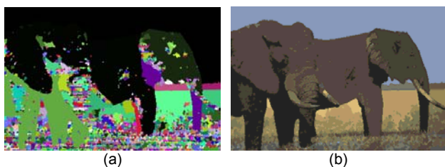
Fig. 11. Oversegmentation and oversegmentation reduction results for the elephants (296059 from the The Berkeley Segmentation Dataset ) test image (384x256 pixels), (a) gradient: pca, threshold 0%, level 6%, catchment basins: 3107, (b) Ward's minimum variance, L1 standardization, attributes: average, 11 classes
