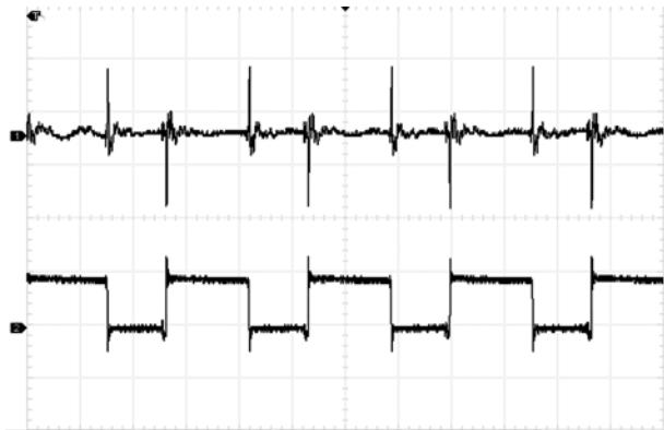
Fig.22. Common mode current (top) and switch node voltage (bottom) in time domain
