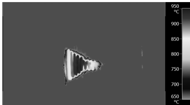
Fig. 3. The temperature field of tungsten coil of lamp, obtained using the three-colour thermal imager [6]
