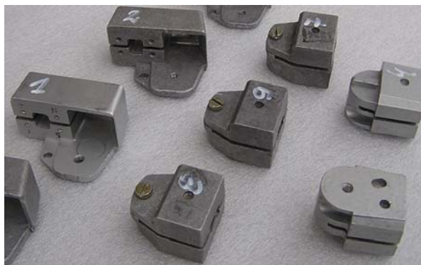
Fig.6. Some kinds of Alnico braking magnets used in induction watt-hour meters
