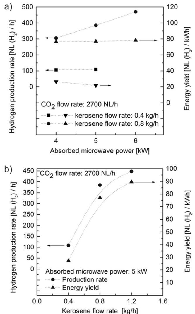
Fig.4. Hydrogen production rate and energy yield of hydrogen production as a function of absorbed microwave power at CO<sub>2</sub> flow rate - 2700 NL/h (a) and as a function of kerosene flow rate at CO<sub>2</sub> flow rate - 2700 NL/h and absorbed microwave power P<sub>A</sub> - 5kW (b).
