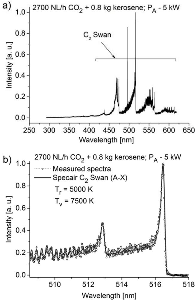
Fig.2. The measured emission spectrum of CO<sub>2</sub> plasma with kerosene vapour addition (a) and the comparison of the measured and simulated emission spectra of C<sub>2</sub> Swan system (b) at CO<sub>2</sub> flow rate - 2700 NL/h, kerosene vapour flow rate - 0.8 kg/h and absorbed microwave power P<sub>A</sub> - 5kW, measured 15 mm below waveguide.
