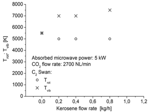
Fig.3. The rotational and vibrational temperatures of the C<sub>2</sub> molecule as a function of kerosene flow rate at CO<sub>2</sub> flow rate - 2700 NL/h and absorbed microwave power P<sub>A</sub> - 5kW, measured 15 mm below waveguide.
