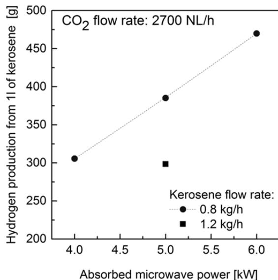
Fig. 5. Hydrogen production from 1 l of kerosene as a function of absorbed microwave power at CO<sub>2</sub> flow rate – 2700 NL/h obtained for two different kerosene flow rate.
