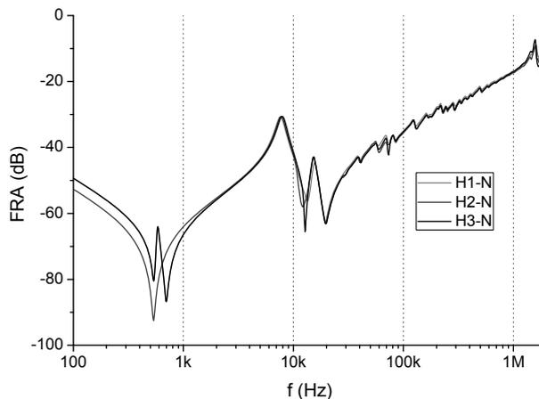
Fig.1. FRA results of transformer TORc 16000/115
