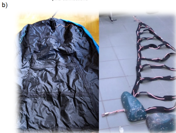
Fig. 3. a) diagram of tent parts connections, b) copper cord mesh after (left) and before (right) mended
