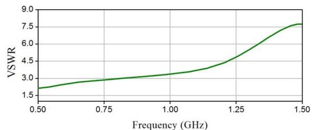
Fig. 2. VSWR curve of rectangular microstrip antenna.
