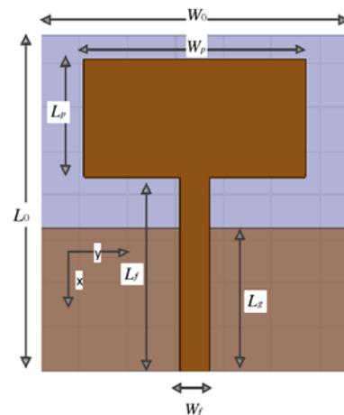
Fig.1. Schematic configuration of rectangular microstrip antenna.
