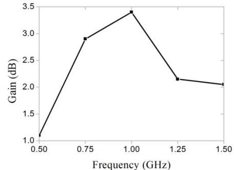
Fig.10. Measured peak gain of the fabricated UWB antenna sensor.
