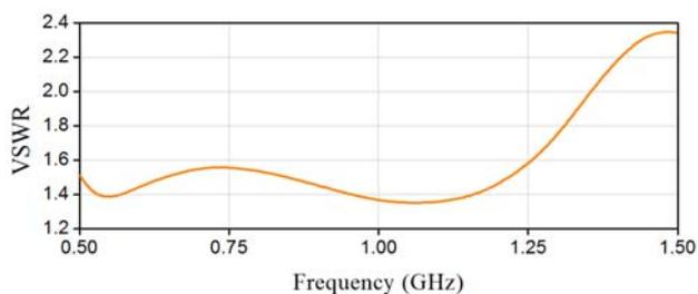
Fig. 4. VSWR curve of antenna after the 1<sup>st</sup> optimization.
