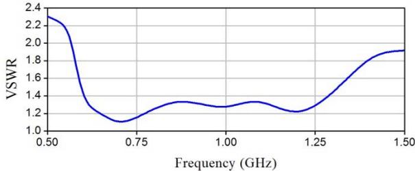
Fig.8. Measured VSWR of the fabricated UWB antenna sensor.
