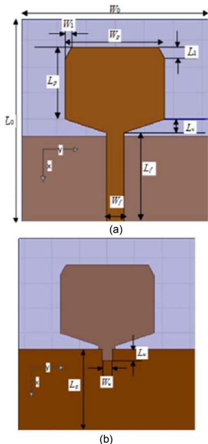
Fig.3. Schematic configuration of antenna after the 1<sup>st</sup> optimization. (a) Top view; (b) Back view.
