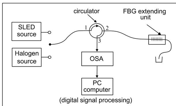
Fig. 1. Scheme of experimental setup for FBG reflected spectra receiving
