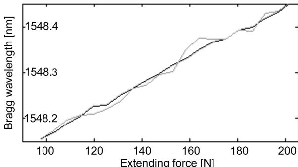
Fig. 3. Sensor processing characteristics received from reference and noisy spectra
