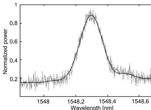
Fig. 2. Comparison of spectra measured with high power and low powered sources
