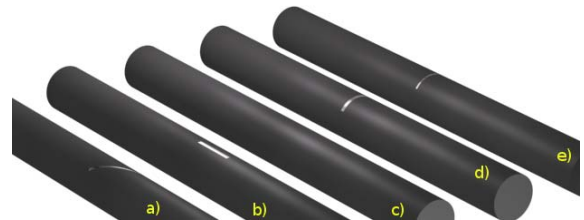
Fig. 5. Defect locations on the rod
