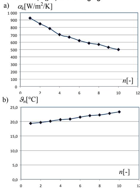
Fig.4. Change in the convective heat transfer coefficient (a) and the water temperature (b) along the channel length (for successive channel zones).
