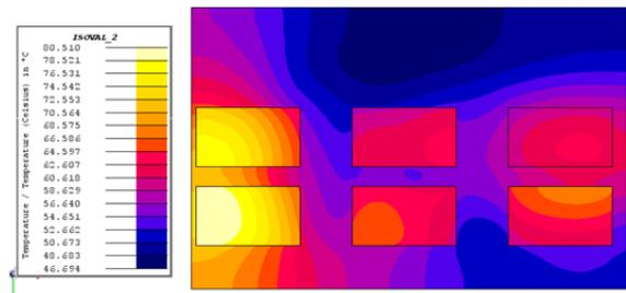
Fig.5. Temperature distribution on the radiator surface and the surfaces representing casings of the IGBT modules, calculated for the convective heat transfer coefficients increased by 20%.
