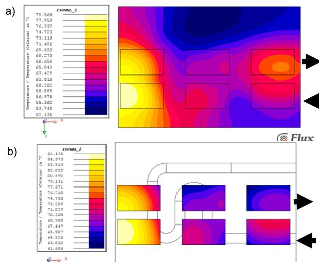
Fig.3. Temperature distribution: a) on the radiator surface, b) on the surface of casings of the IGBT modules cooled.
