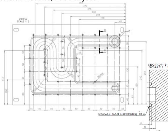
Fig.1. Water-cooled radiator, the water channel view.
