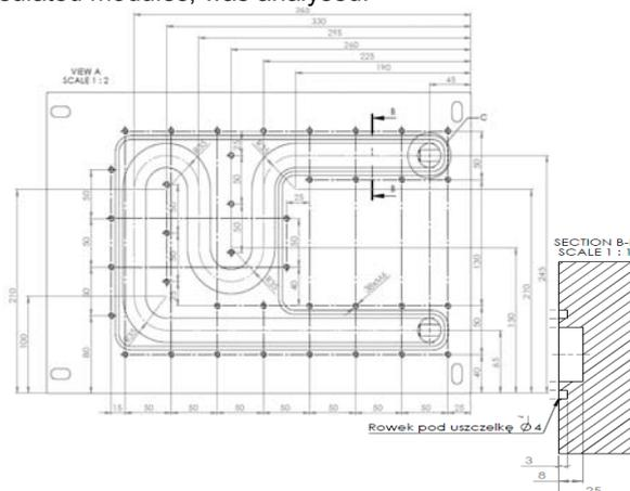
Fig.1. Water-cooled radiator, the water channel view.
