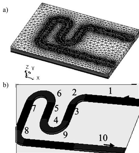
Fig.2. The 3D calculation model of a radiator: a) discrete model; b) division of the channel into ten zones with different temperatures of the cooling water.
