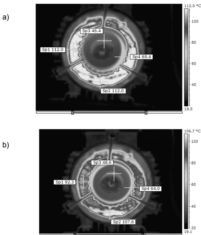
Fig.2. Temperature distribution in face part of inductor windings in course of electromagnetic mill operation: a) without cooling ( t=6 minutes, I=13 A), b) with cooling ( t=16 minutes, I=13 A)
