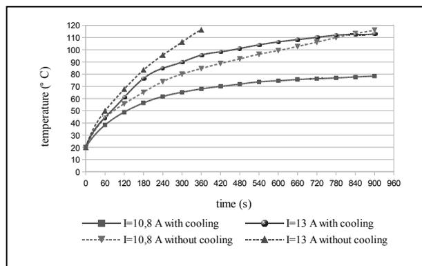
Fig.3. Temperature distribution in face part of inductor windings in course of electromagnetic mill operation with and without cooling for inductor current of 10,8 A and 13 A
