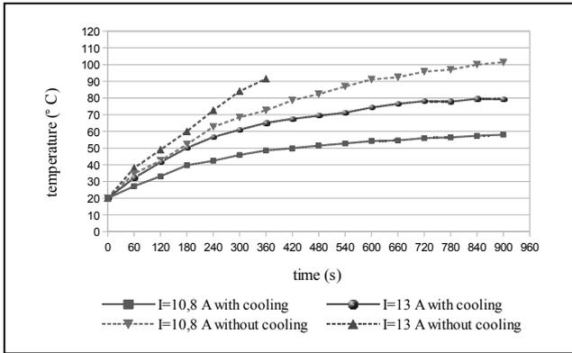
Fig.4. Maximum temperature distribution in the inductor magnetic core in course of electromagnetic mill operation with and without cooling for inductor current of 10,8 A and 13 A
