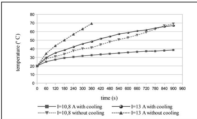
Fig.5. Maximum temperature distribution in the working chamber in course of electromagnetic mill operation with and without cooling for inductor current of 10,8 A and 13 A
