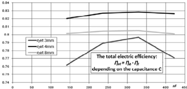
Fig. 9. The graph presents the dependence of the total electric efficiency of the inverter model on the capacity  $C$  installed in the output oscillatory circuit
