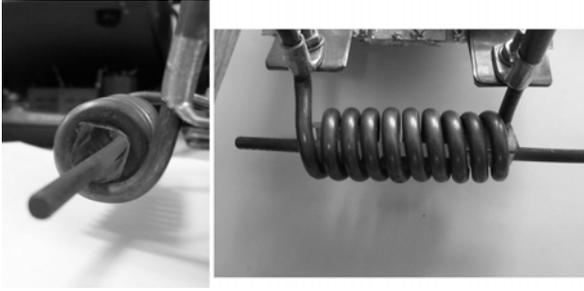
Fig. 6. The inductor with a sample load (steel rod Ø4 mm) during the heating process
