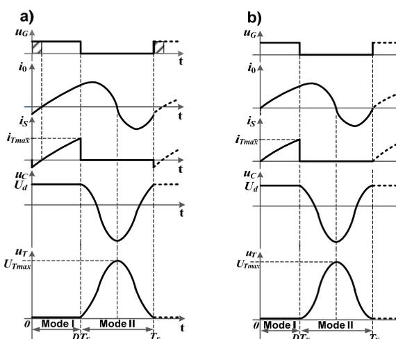
Fig. 3. Current and voltage waveforms in the inverter under ZVS operation: a) suboptimum operation; b) optimum operation;  $u_G$  – gate signal,  $i_0$  – load current,  $i_s$  – switch current,  $u_c$  – voltage across the capacitor,  $u_T$  – voltage across the switch
