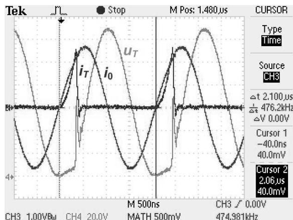
Fig.5. Waveforms of the load current  $i_0$  (25 A/div), the transistor voltage  $u_T$  (20V/div) and transistor current  $i_T$  (25 A/div) in a model of the inverter with steel load inside the inductor:  $U_d = 59$  V,  $C = 0.329$   $\mu$ F
