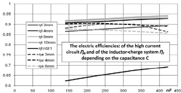
Fig. 8. The graph presents the dependence of the electric efficiencies of: electrical power circuit ( $\eta_e$ ) and heating system ( $\eta_t$ ) of the inverter model on the capacity  $C$  installed in the output oscillatory circuit
