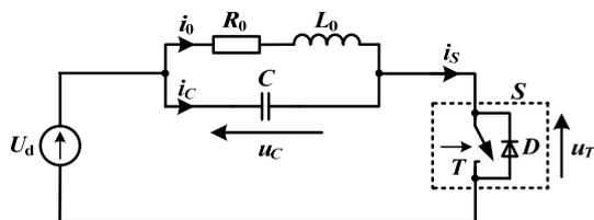
Fig. 1. Circuit diagram of the single-switch inverter
