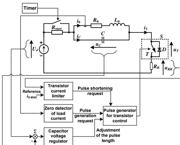
Fig.4. Block diagram of the inverter control system
