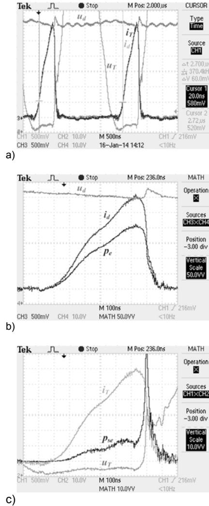
Fig.7. Examples of supply current waveforms  $i_d$ , voltage waveforms  $U_d$ , the current in transistor  $i_T$ , voltage on transistor  $U_T$ , input power  $p_e$  and power losses on transistor  $p_{se}$  in system with example load: ferromagnetic steel rod Ø3 mm, with capacitor  $C = 329$  nF, at a supply voltage  $U_d = 70.6$  V:
