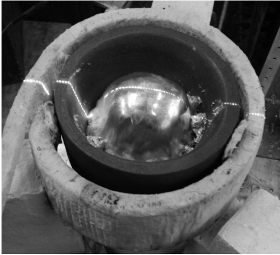
Fig. 1. Measurement site with ceramic crucible and liquid aluminium
