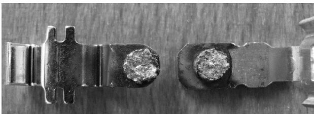
Fig. 4. Exemplary photograph of current path with AgCdO10 switching device contacts after tests
