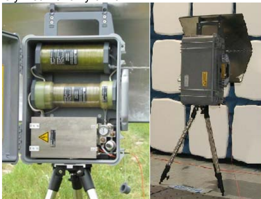
Fig.2. Suitcase system for generation pulses Diehl DS110F
