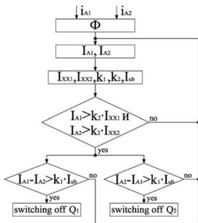
Fig. 1. Operation algorithm of protection of two parallel lines for phase A.
