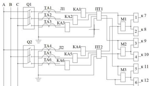
Fig. 2. Connection diagram of measuring elements of two parallel lines protection.
