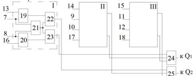
Fig. 3. Principle diagram of the logical part of protection of two parallel lines without voltage path.
