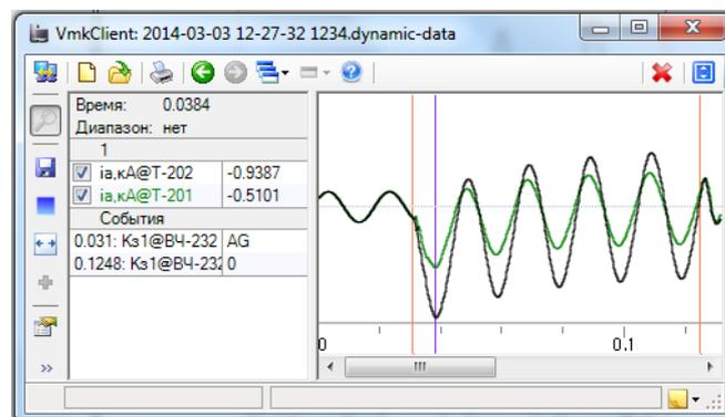
Fig. 4. Oscillograms of phase A currents of the first and second lines under one-phase SC on the first line.
