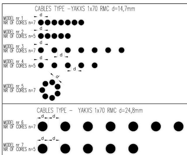
Fig. 2. Spatial configuration of the wires
