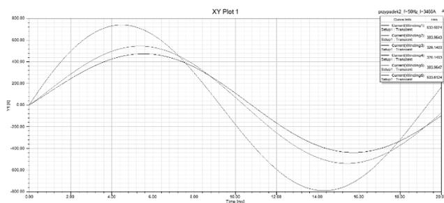
Fig.5. The time dependence of wire load
