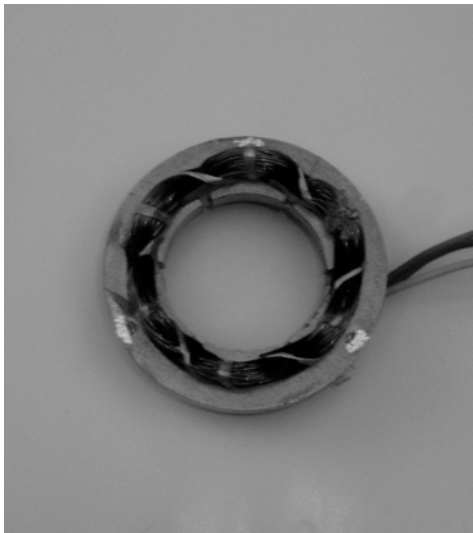
Fig. 3. View of the stator with coils
