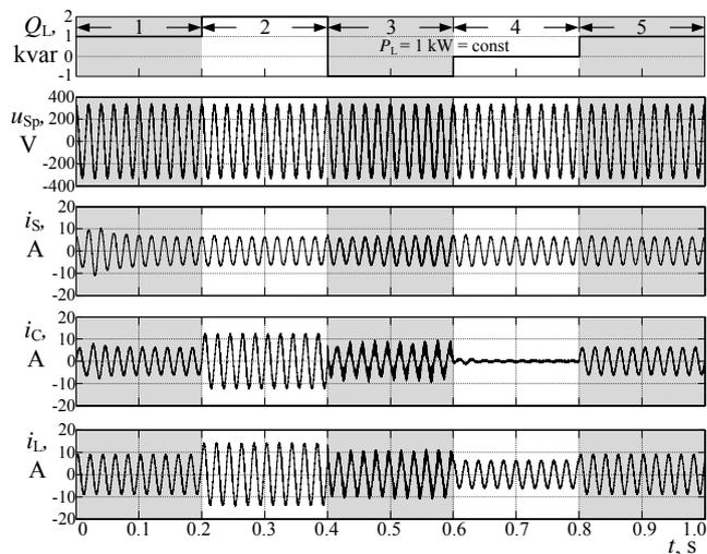
Fig. 9. Current waveforms:  $i_s$ ,  $i_c$ ,  $i_L$  and  $u_{Sp}$  voltage waveform for whole sequence of load reactive power changes (1+5)
