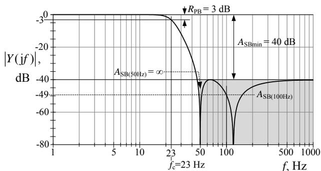
Fig. 6. Magnitude of frequency response of selected filter
