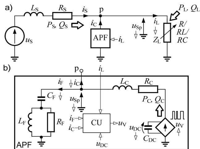
Fig. 4. A simplified model of single-phase power system with the APF, a) location of the APF in the system, b) macromodel of the APF
