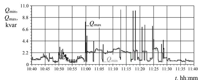
Fig. 3. An example of the maximum and the minimum value ( $Q_{max}$ ,  $Q_{min}$ ) of reactive power during one hour
