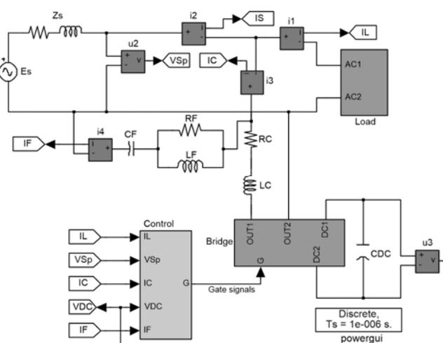
Fig. 8. Single-phase system with APF in Matlab-Simulink
