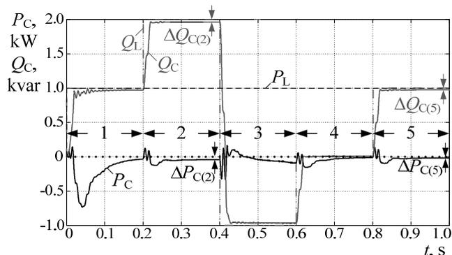
Fig. 10. Waveform of active power  $P_C$  and reactive power  $Q_C$  of the APF in states 1÷5
