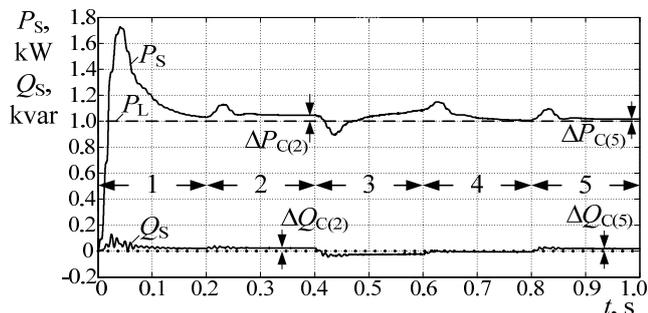
Fig. 11. Waveform of active power  $P_S$  and reactive power  $Q_S$  of source in states 1÷5
