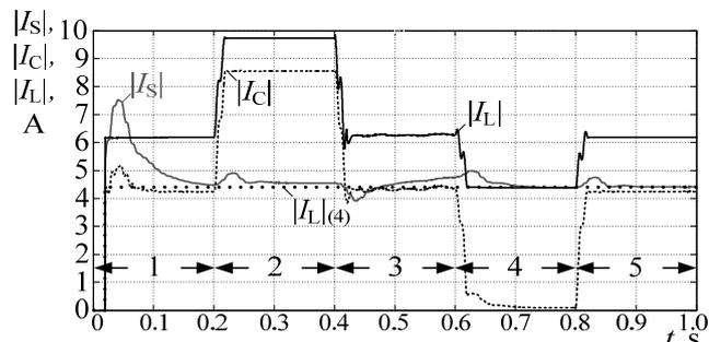
Fig. 12. Changes of RMS value of currents: source  $|I_S|$ , load  $|I_L|$  i APF  $|I_C|$  in states 1÷5
