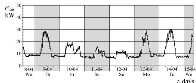
Fig. 1. Average total active power for the measured building in 1 week period
