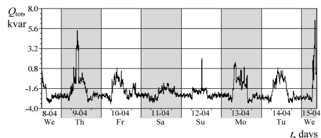
Fig. 2. Total average reactive power  $Q_{tot}$  for the measured building in 1 week period
