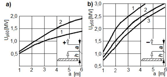
Fig. 6. Influence of point electrode polarity on the point-plate and point-point grounded electrode arrangement
