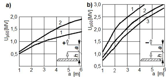
Fig. 6. Influence of point electrode polarity on the point-plate and point-point grounded electrode arrangement
