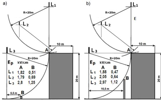
Fig. 4. Values of field modules caused, by different position of leaders, at the apex point of a structure and protected external element being in the horizontal distance of: a) 6,5 m and b) 16,5 from the leader
