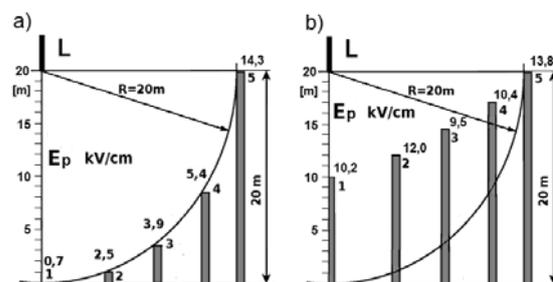
Fig. 3. Comparison of field modules at the tops of vertical rods: a) reaching the surface of rolling sphere, b) incoming into the sphere
