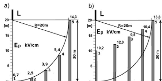
Fig. 3. Comparison of field modules at the tops of vertical rods: a) reaching the surface of rolling sphere, b) incoming into the sphere
