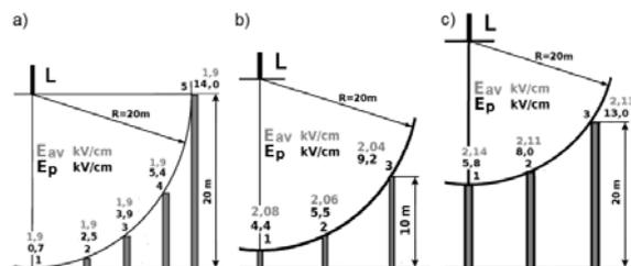
Fig. 2. Comparison of field modules  $E_p$  at the tops of vertical rods, distributed along the rolling sphere surface, with average values  $E_{av}$  of the field between these tops and leader head placed on the height: a) 20 m, b) 22, c) 31 m. .
