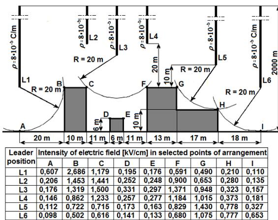
Fig. 5. Distribution of field modules caused by different leaders at the apex points of structure arrangement
