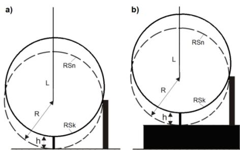
Fig. 7. Graphical explanation of the correction of protected zone range created by vertical air termination positioned: a) on the ground surface, b) on the building roof; RSn - the rolling sphere placed by RSM, RSk – rolling sphere in corrected position.
