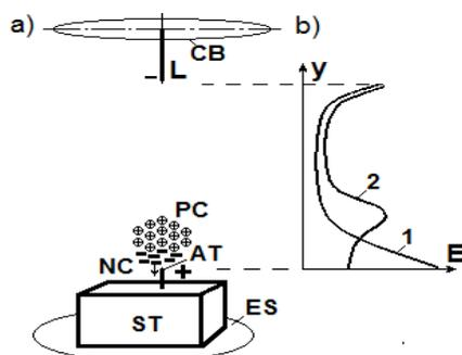
Fig. 8. Illustration: a) arrangement leader (L)-air termination (AT) and b) electric field intensity distribution (E) in this arrangement; PC - positive space charge, NC - vanished electrons into AT, CB – thunderstorm cloud base, ST – structure, ES – earth surface, Curves 1 and 2 - field distribution before and after the ionization and space charge appearance
