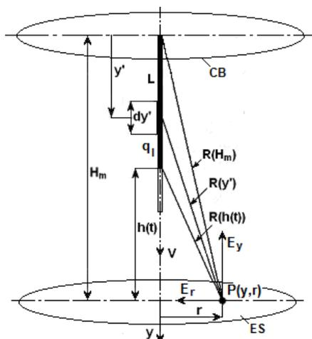
Fig. 1. The model of arrangement adopted to investigations; L - leader aiming at the point  $P(y,r)$  positioned on or above the ground surface (ES);  $y, r$  - coordinates of arrangement, CB- thunderstorm cloud base, L - leader,  $q_l$  - linear density of leader charge,  $v$  - leader development velocity,  $H_m$  - height of the thunderstorm cloud base,  $h(t)$  - the height of the leader head.
