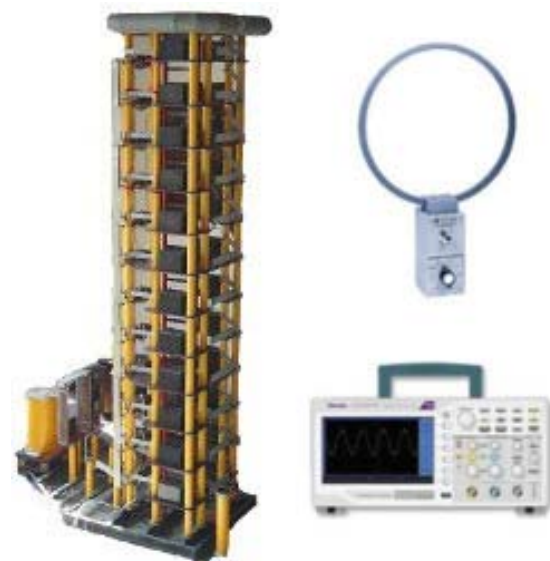
Fig. 4. High voltage surge generator 2.4 MV, passive loop antenna EMCO model 6509 and oscilloscope Tektronix TBS1052-EDU.
