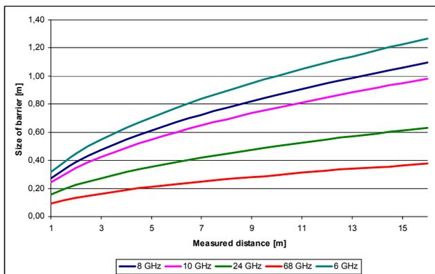
Fig. 8. Size of barrier depended on frequency of level gauge
