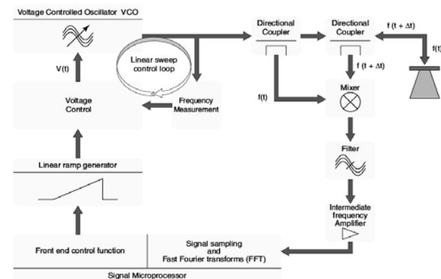
Fig. 1. Standard block diagram of FM-CW level gauge [2]
