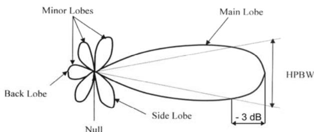
Fig. 3. Antenna radiation pattern
