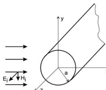
Fig. 6. Circular cylinder – plane wave incidence
