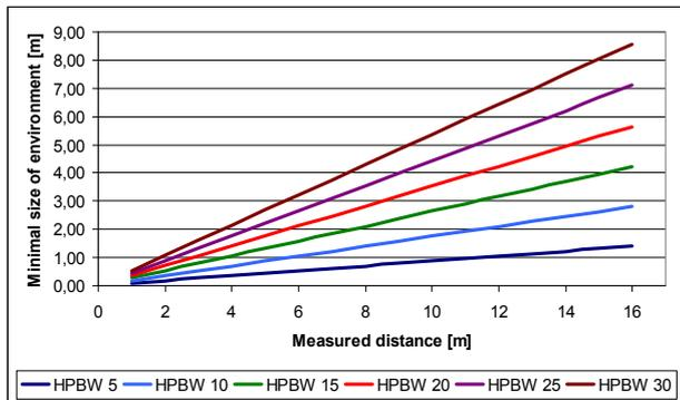
Fig. 7. Minimal dimensions of laboratory with consider of antenna's HPBW
