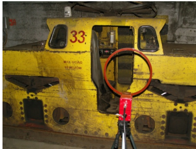
Fig. 4. Traction locomotive, loop antenna for magnetic field measurements in front.
