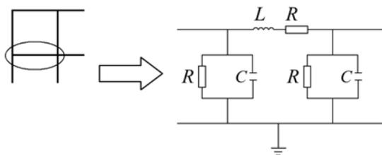
Fig.2. Simplified mesh branch model
