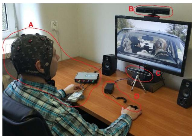
Fig.1. The developed system, A - EEG, B - Kinect, C - eye tracker, D - GSR
