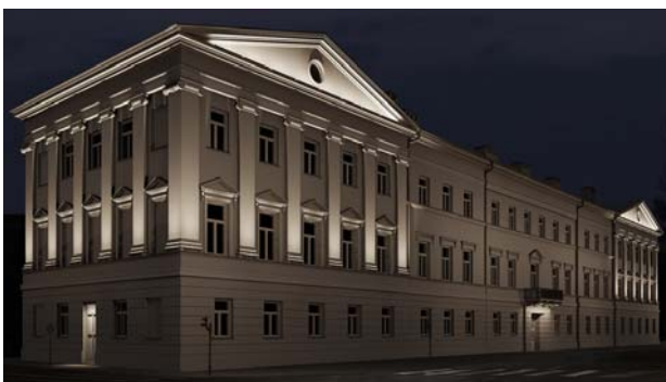
Fig. 4. Floodlighting option II - mixed method with emphasis of tympanums and pilasters in the side breaks in walls
