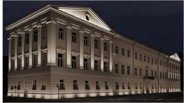
Fig. 5. Floodlighting option III – mixed method with emphasis tympanums, pilasters in the side breaks in walls and elevation of the ground floor
