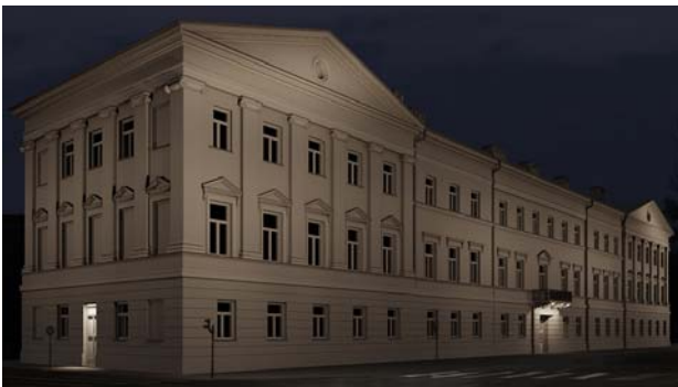
Fig. 3. Floodlighting option I – flood method
