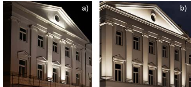
Fig. 6. Differences between floodlighting field trials (a) and a computer simulation (b)
