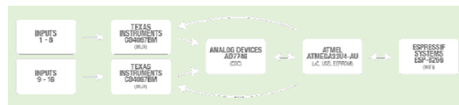
Fig. 2. Block diagram of data acquisition module
