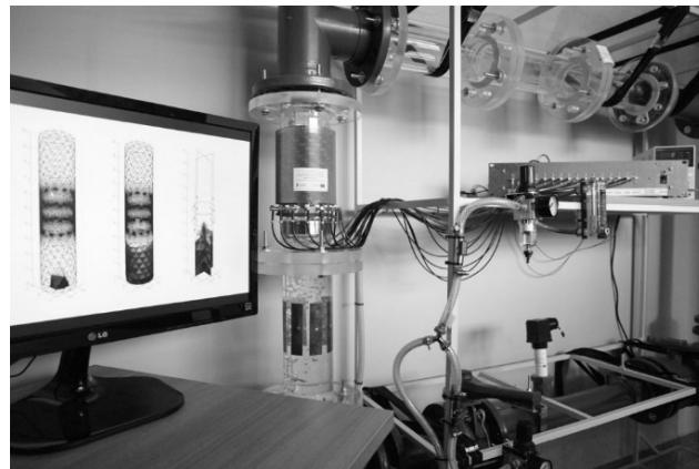
Fig.8. The laboratory model of the pipeline tomography system
