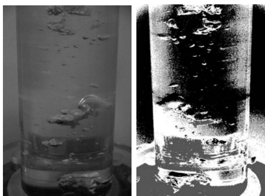
Fig. 17. Genetic algorithm: 5 classes, populations 8000, a filter for noise removal pepper and salt
