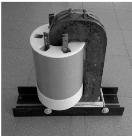
Fig.3. The model of the copper transformer Cu with a capacity of 10 kVA [16].
