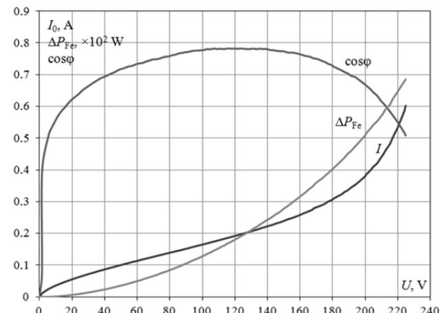
Fig. 8. The characteristics of no-load status of 13.8 kVA transformer
