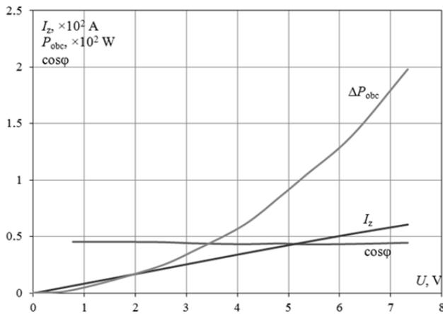
Fig. 9. The characteristics of no-load status of 13.8 kVA transformer.
