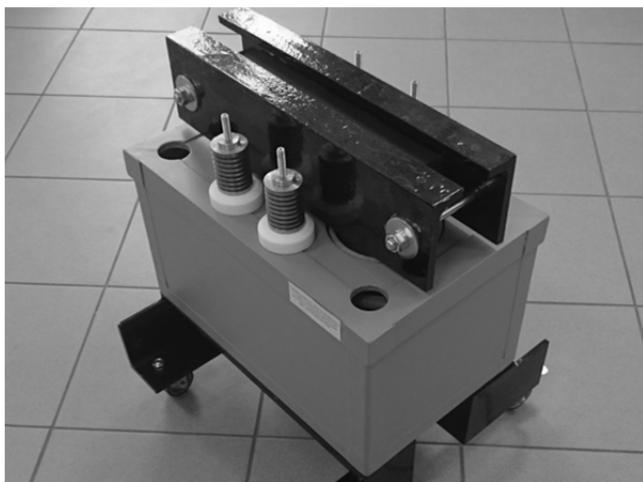
Fig. 3. 15 kVA superconducting transformer
