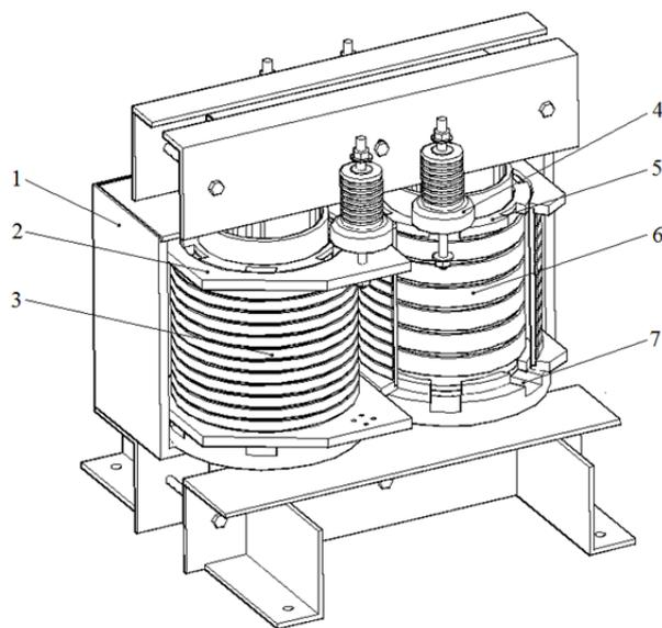
Fig. 4. Outline cross-section of the design: 1 - cryostat, 2 - HV carcass, 3 - HV winding, 4 - bushings current, 5 - LV carcass, 6 - LV winding, 7 - cooling ducts
