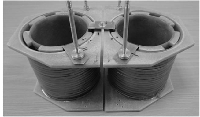
Fig. 7. Windings in carcasses
