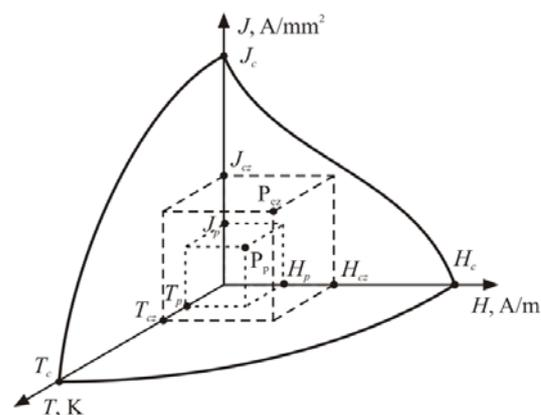
Fig. 2. Critical surface of the superconductor [6] [7]
