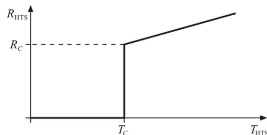
Fig. 1. A simplified characteristics of the superconductor transition [6] [7]
