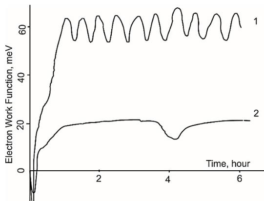
Fig.11. Variation of the integral value of rubbing surface work function with time for some materials (1 – brass 37-63; 2 – stainless steel 12X18H10T at load 0.12 MPa. In these case an initial values of electron work function zeroed for both metals
