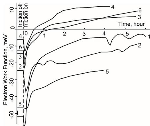
Fig.10. Variation of the integral value of rubbing surface work function with time for some materials (1 – brass; 2 – bronze (Al); 3 – bronze (Sn); 4 – commercial copper; 5 – stainless steel; 6 – medium carbon steel) at load 0.05 MPa
