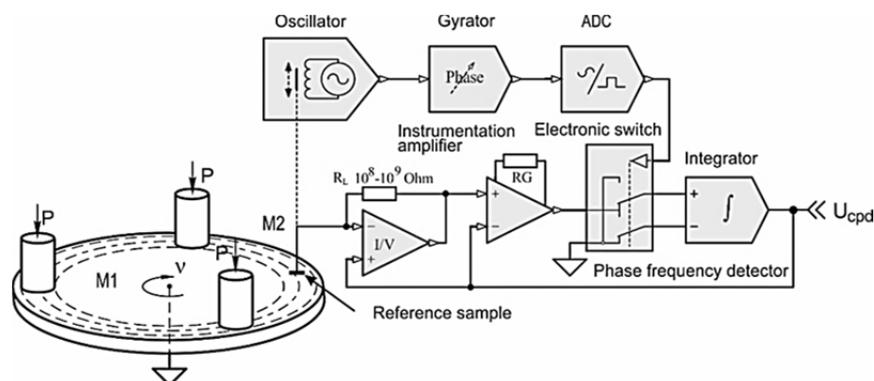
Fig.1. Functional diagram of the system for friction processes monitoring on the electron work function with the Kelvin-Zisman probe
