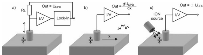
Fig.2. Charge sensitive techniques measurement principle: a) The Kelvin-Zisman capacitor, b) the Non-vibration capacitor and c) the Ionization capacitor
