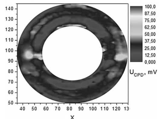
Fig.9. The contact potential difference distribution on friction surface of the steel sample at the normal pressure of 0.025 MPa registered by Scanning Kelvin-Zisman probe
