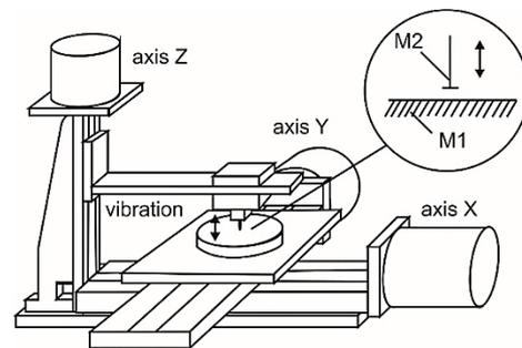
Fig.4. The schematic diagram of the Scanning Kelvin-Zisman probe
