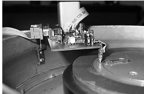
Fig.3. The modification of the Non-vibration probe for friction testing
