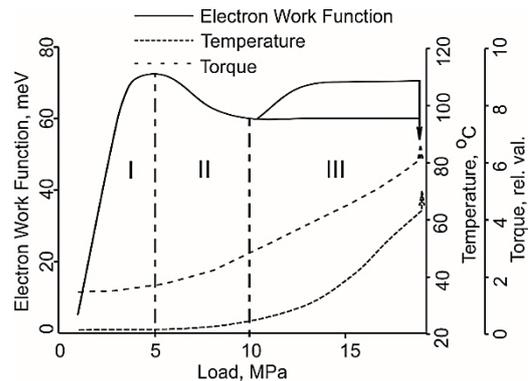
Fig.7. Bronze rubbing surface electron work function, torque and surface temperature vs. normal load curves
