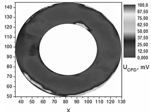
Fig.8. The contact potential difference distribution on steel sample initial surface registered by Scanning Kelvin-Zisman probe
