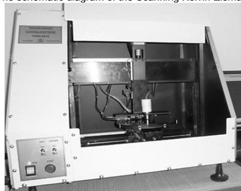
Fig.5. The modification of the Scanning Kelvin-Zisman probe device for testing of the electron work function (or contact potential different) distribution
