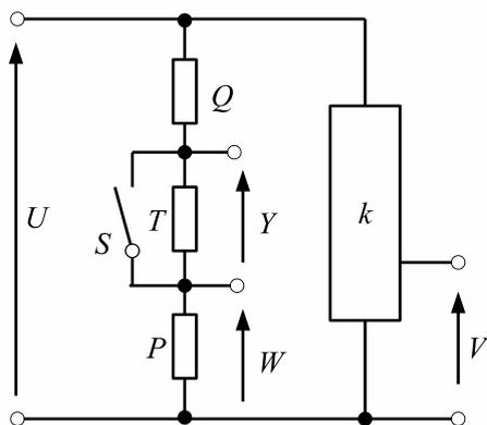
Fig.2. Schematic diagram of an adaptive high voltage divider
