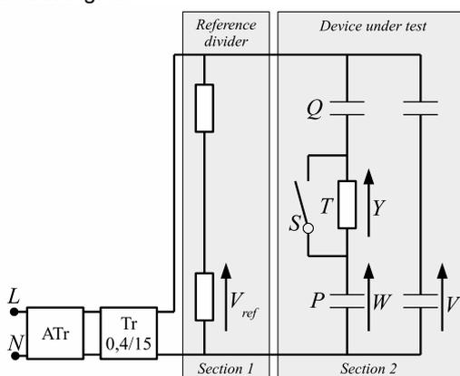
Fig.3. Laboratory setup used in experiments (tested divider represented in detail)
