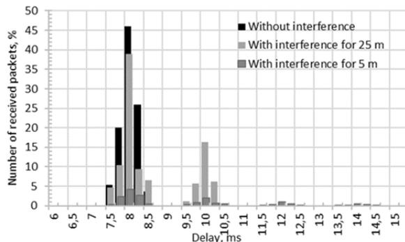
Fig.6. Delay histogram for IEEE 802.15.4 under and without Wi-Fi interference for distance of 5 meters between Wi-Fi and ZigBee
