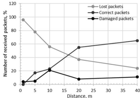
Fig.4. PRR for IEEE 802.15.4 under IEEE 802.11 interference
