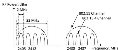
Fig.2. Transmission channels for IEEE 802.11 and 802.15.4
