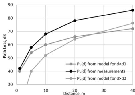
Fig.7. Path loss from measurements and model
