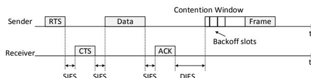
Fig. 1. Messages and delays defined in the 802.11 MAC protocol
