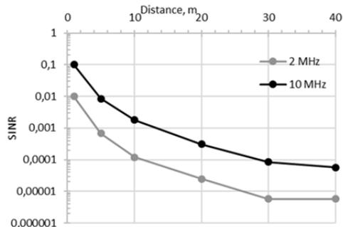
Fig.5. SINR versus distance and frequency shift of Wi-Fi channels from ZigBee transmission channel
