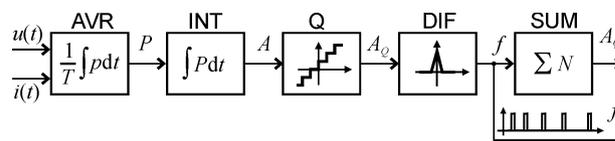
Fig.2. Functional diagram of the static electricity meter
