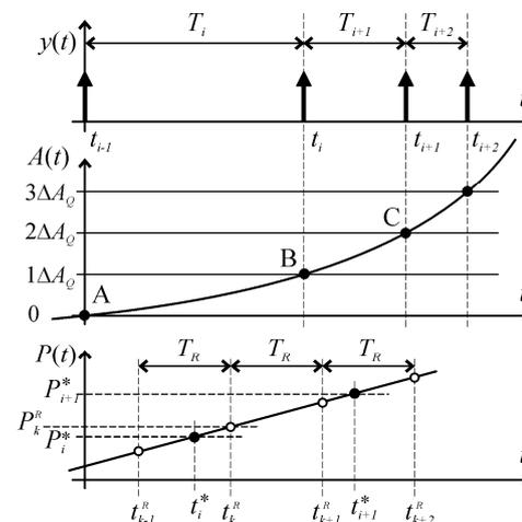
Fig.5. Approximation of active energy  $A(t)$  with a second-degree polynomial between the three successive pulses [10]
