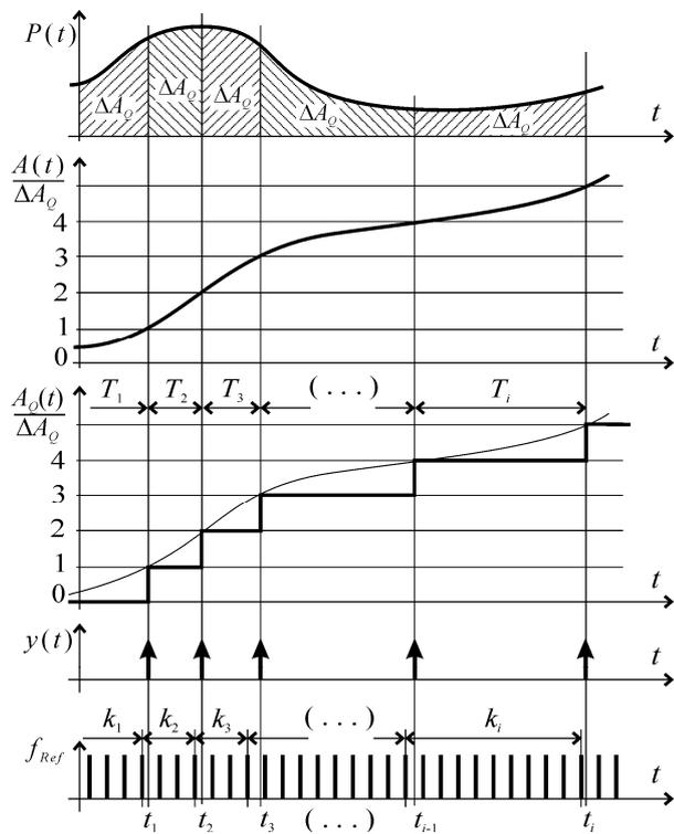
Fig.3. Time courses of signals in the static electricity meter
