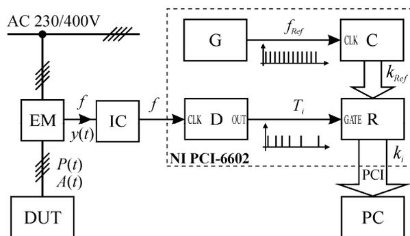
Fig.7. Block diagram of the measurement system with electricity meter working as transducer of active power to frequency
