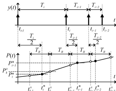
Fig.6. Approximation of instantaneous active power  $P(t)$  with a first-degree polynomial between the two adjacent points [10]
