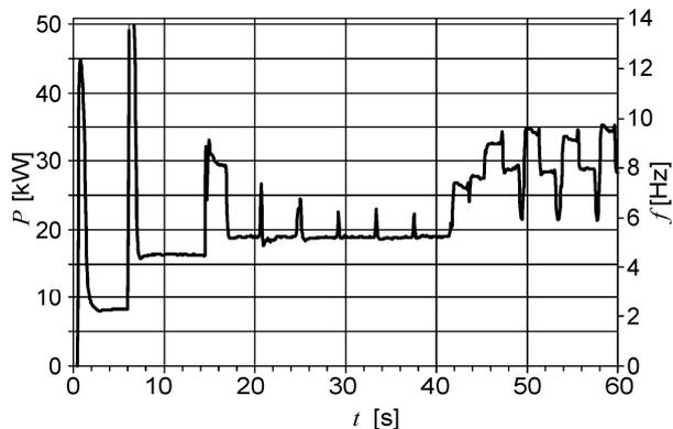
Fig.9. Active power determined on the basis of the test signal of the static electricity meter
