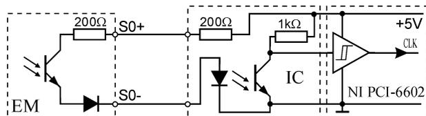
Fig.8. Current interface S0 for transmitting pulses from the electricity meter EM through the interface circuit IC to DAQ-Card
