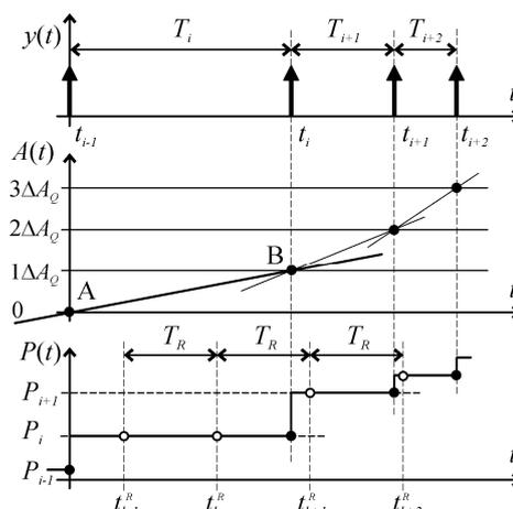
Fig.4. Approximation of instantaneous active energy  $A(t)$  with a first-degree polynomial between the two adjacent pulses [10]
