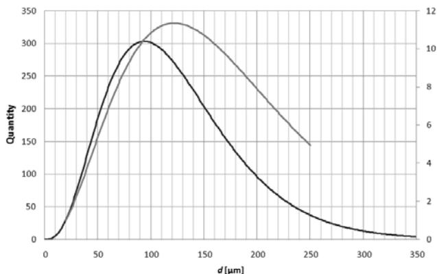
Fig.3. Experimentally obtained distributions of diameters of aerosol droplets in the air (the black line, left scale) and adhering to the recorder's plate (the grey line, right scale)
