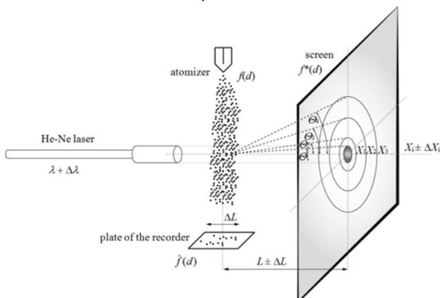
Fig.2. A scheme of the experiment in which water aerosol was directed onto the laser beam causing light scattering on the droplets and producing on the screen a diffraction image whose minima allow one to determine the size of the droplets
