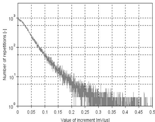
Fig. 9. Incremental decomposition of signal while 2 A arcing
