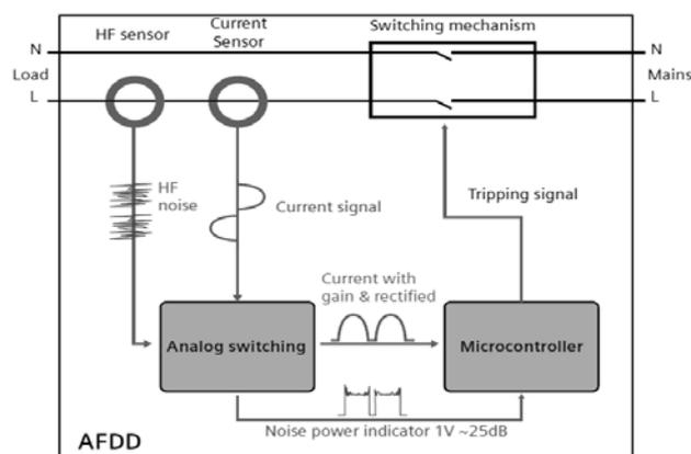
Fig. 1. Block diagram of the Siemens 5SM6 detector [19]
