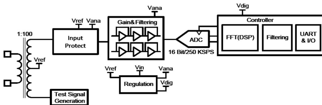
Fig.2. Block diagram of the Texas Instruments RD-195 detector [20]
