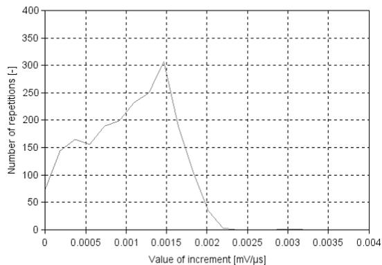
Fig. 6. Incremental decomposition of signal while non-arcing
