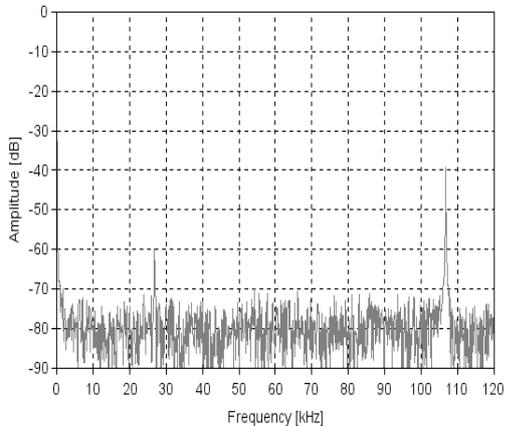
Fig. 4. Frequency spectrum of signal measured while non-arcing
