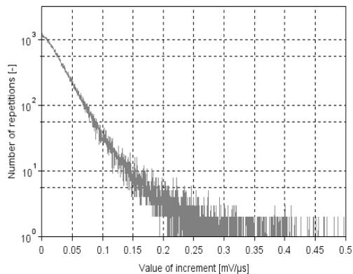
Fig. 8. Incremental decomposition of signal while 0.5 A arcing
