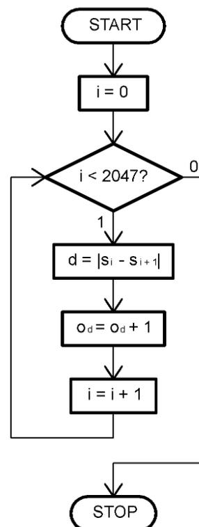
Fig. 3. Algorithm of the incremental decomposition calculation
