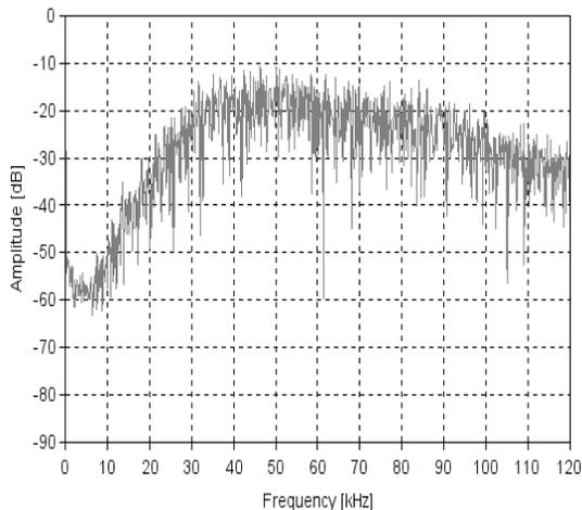
Fig. 5. Frequency spectrum of signal measured while arcing
