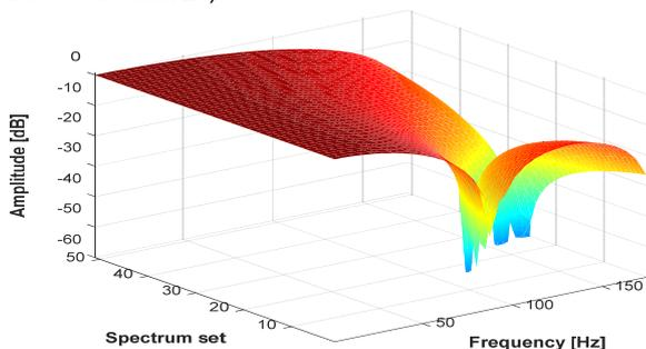
Fig. 8. Frequency spectra of modified Quadratic Spline scaling function (original spectrum at index 25)
