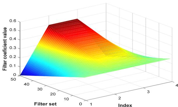
Fig. 7. Modifications of Quadratic Spline scaling function (original filter set at index 25)
