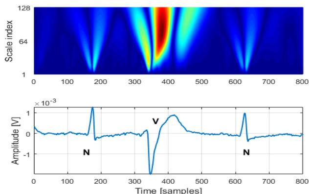
Fig. 4. A sample type V QRS complex (the middle ECG cycle) taken from the database [5] together with CWT results computed for 128 scales and with a use of *Quadratic Spline* wavelet
