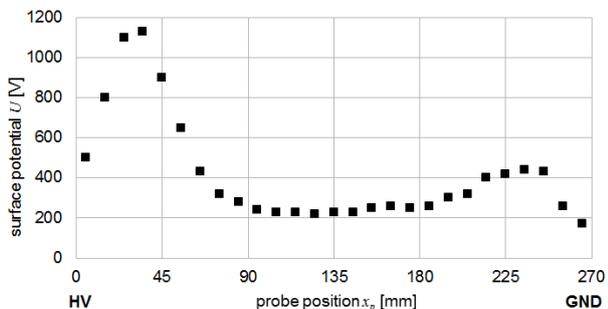
Fig. 3. Surface potential distribution measured after positive impulse flashover ( $U_f = +201.5$  kV). HV and GND refer to high voltage and grounded fittings respectively. Model: EG-LSR
