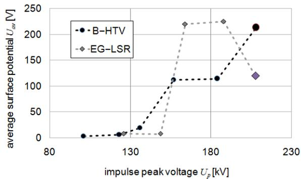
Fig. 7. Average value of the surface potential as a function of impulse voltage  $U_p$ . Points for highest voltages - for flashover.
