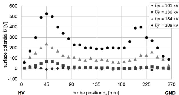
Fig. 5. Surface potential distributions measured after applying positive impulse voltage with ( $U_p$ ) and without ( $U_f$ ) flashover occurrence. HV and GND refer to high voltage and grounded fittings respectively. Model: B-HTV
