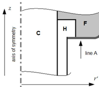
Fig. 10. Close-up of the fitting with defined line along which was calculated field distribution. C – core, H – housing, F – fitting
