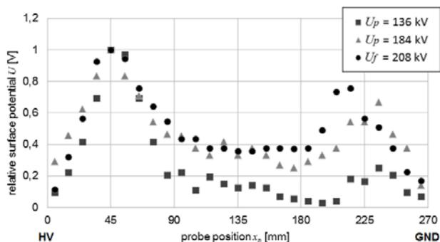
Fig. 6. Relative (related to the maximum value) surface potential distributions measured after applying positive impulse voltage with ( $U_p$ ) and without ( $U_f$ ) flashover occurrence. HV and GND refer to high voltage and grounded fittings respectively. Model: B-HTV
