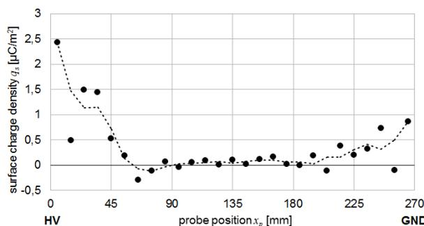
Fig. 4. Surface charge density distribution measured after positive impulse flashover ( $U_f = +201.5$  kV). HV and GND refer to high voltage and grounded fittings respectively. Sample: EG-LSR
