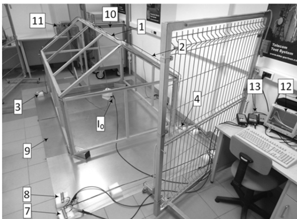
Fig. 2. The laboratory test stand: 1-4, 7-10, I_0 – as in Fig. 1, 11 – injection transformer, 12 – digital oscilloscope, 13 – current probes
