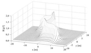
Fig. 6. Module of the magnetic flux density
