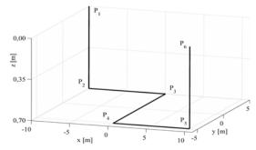
Fig. 5. Route of underground cable line with complex geometry
